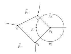
The Voronoi diagram is a graph on vertex set of Voronoi points with some unbounded edges. In this figure,  $v_1$  is the center of a circle containing  $p_1, p_2, p_3$  in its boundary. This circle cannot contain any input point on its interior.
