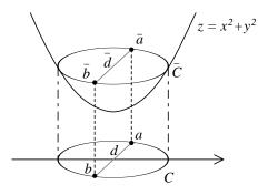
Downward facing facets of  $CH(\bar{P})$ , Lower Hull:  $LH(\bar{P})$ , correspond to the simplices in the Delaunay triangulation.
